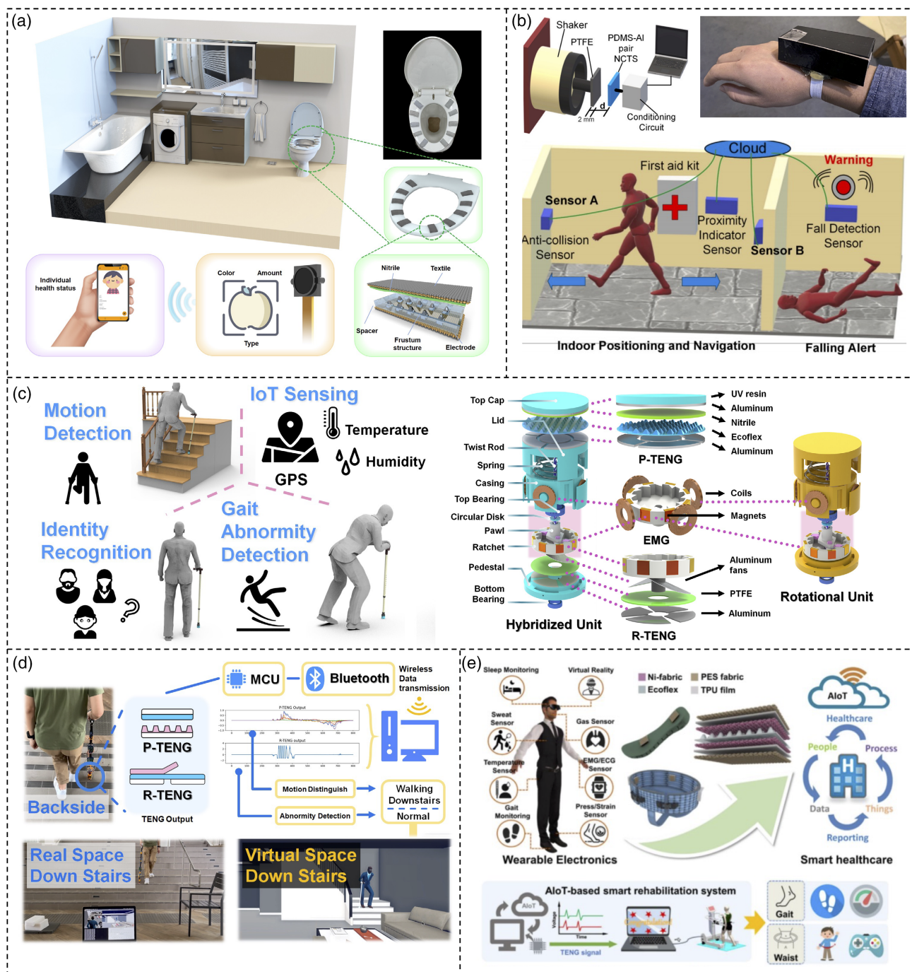
Figure 8. Self-sustainable system for application of smart home. a) A low-cost T-TENG pressure sensor integrated with vision sensor aiming for an AI-Toilet. Reproduced with permission. [235] Copyright 2021, Elsevier. b) A contactless tracking for elderly and visually impaired people in the home achieved by noncontact TENG sensors. Reproduced with permission. [236] Copyright 2021, Elsevier. c) A multifunctional walking stick aiming for the caregiving of elderly and motion-impaired people. Reproduced with permission. [237] Copyright 2021, American Chemical Society. d) Demonstration for the application of indoor monitoring with the caregiving walking stick. e) Schematics of the AIoT-based smart rehabilitation system with gait detection and waist motion capture. Reproduced with permission. [271] Copyright 2021, Wiley-VCH.
